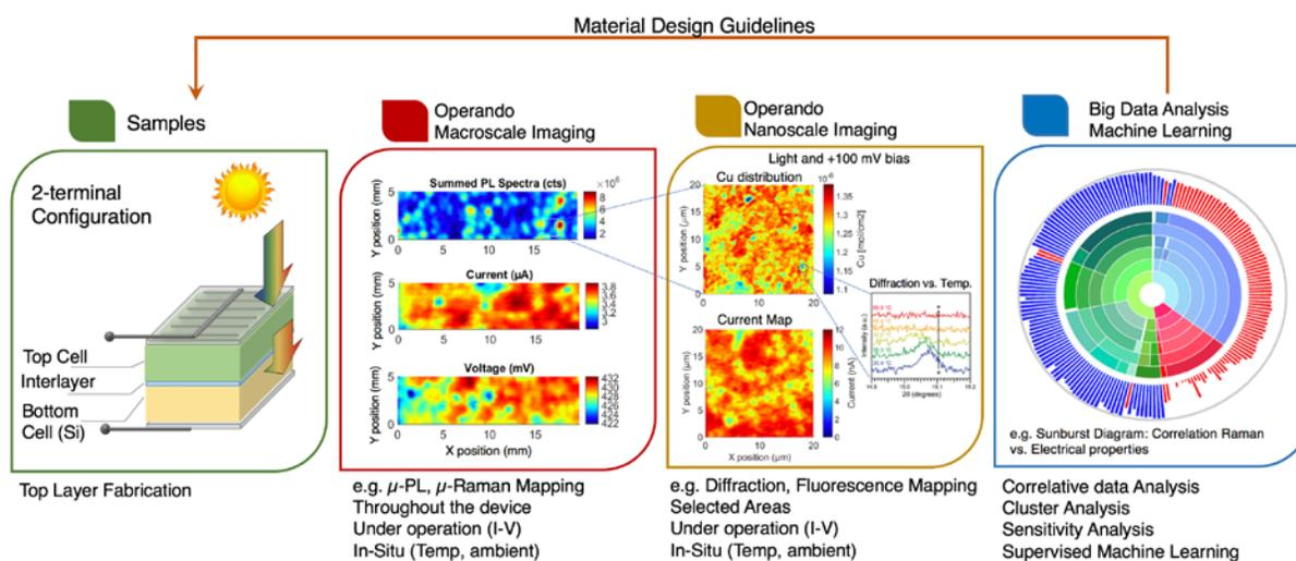
Figure 2. Schematics of a machine learning driven approach to material's design for discovery and engineering of next generation solar cell materials. Data from multiple imaging modalities at different scales can be analyzed to develop guidelines for growth and/or processing of a material. \*Diffraction pattern and sunburst diagram from {Schelhas:2016hc} {Kusne:2015ct} respectively.
