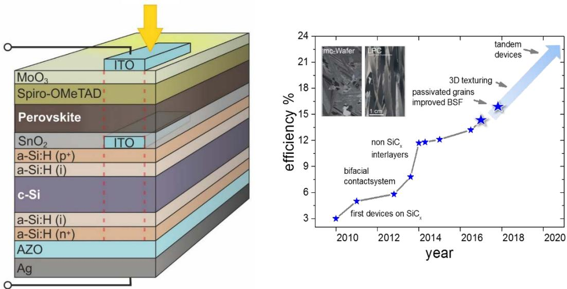
Figure 1: a) Schematic illustration of a monolithic perovskite/silicon heterojunction tandem solar cell. b) Efficiency progress for liquid phase crystallized silicon on glass & roadmap.
