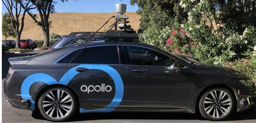
**Figure 2: Autonomous driving vehicle using Apollo platform**
