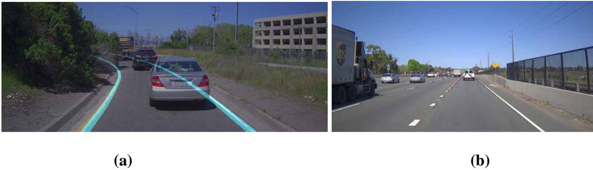
**Figure 5: Example of automated labeling of lane lines (a) Hidden lane lines are labeled (b) 3D lane lines are labeled.**
