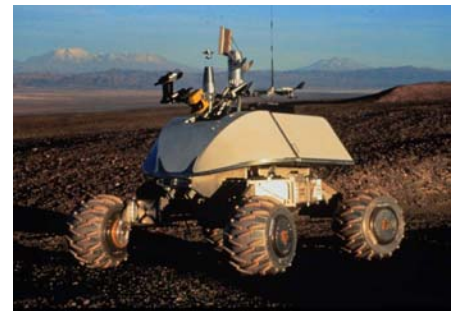
Fig. 1 NOMAD – CMU/NASA gasoline powered robot, from Nomad, 2004. Used by permission
