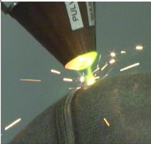
In order to make parts with overhangs, directed energy deposition systems need to either use a 5-axis deposition system (so that material can be deposited from any orientation) or a secondary support material. As these systems are typically used to make metal parts or metal/ceramic composite structures, any supports that are used require machining to remove them.
