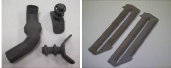
Figure 3. Examples parts of PEAK materials processed via SLS
