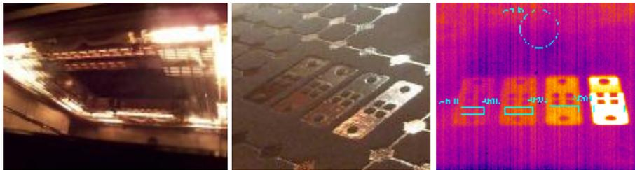
Figure 2. MZ heating (left), SLS part bed (center), same parts seen via infrared thermography during laser scanning (right)
