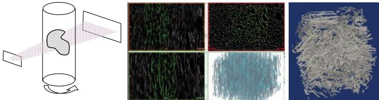
Micro-CT inspection of AM materials; schematic (left), slide data (center), 3D reconstructed AM fibers (right)
