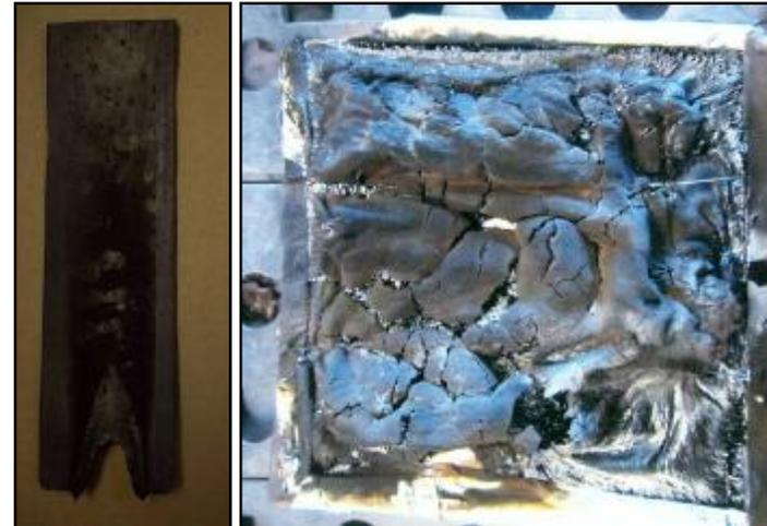
Examples of flammability test coupons
