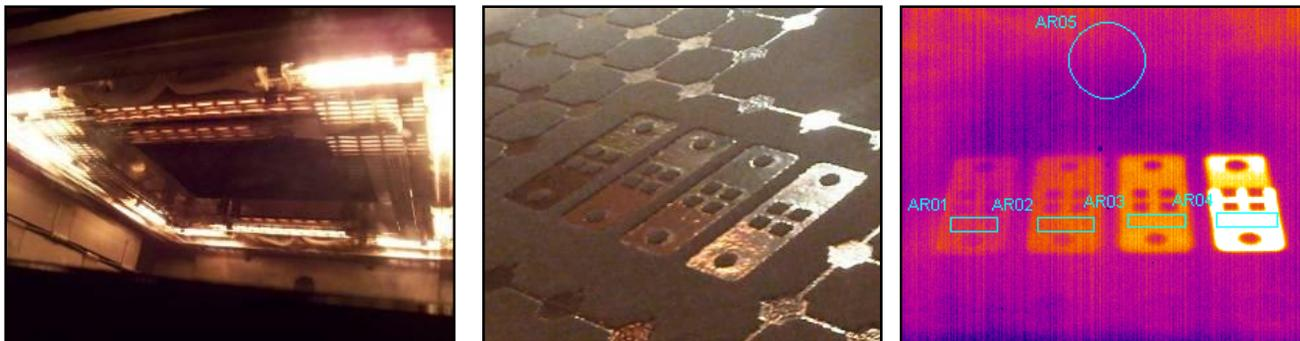
MZ heating (left), SLS part bed (center), same parts seen via infrared thermography during laser scanning (right)
