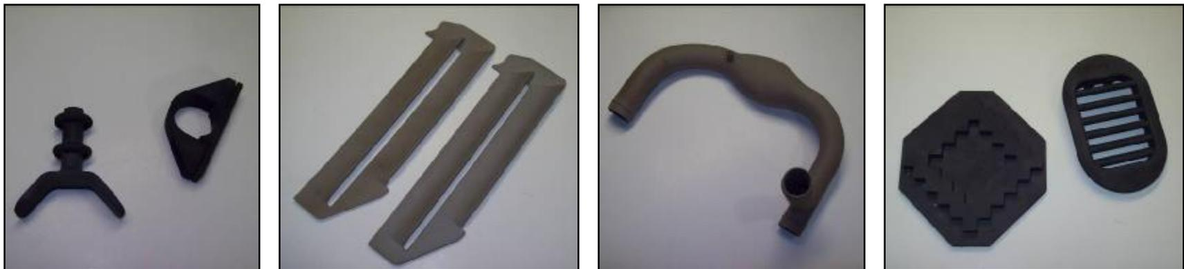
Range of test parts from SLS process, shown in a variety of materials
