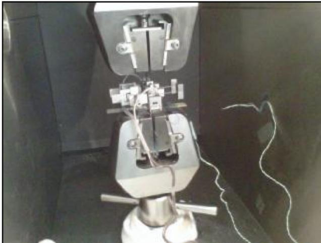
Instrumented, high temp mechanical test cell
