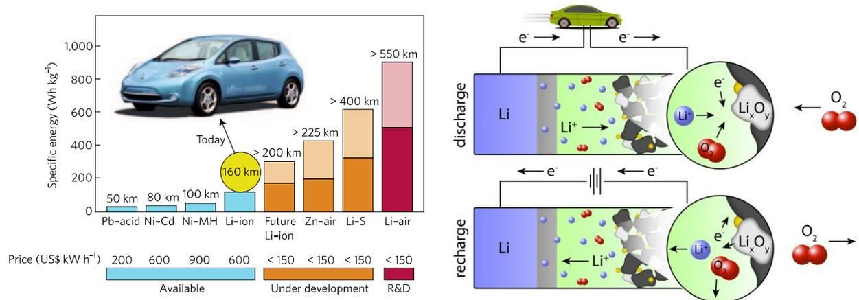
**Fig. 1:** (left) Specific energies for present and future battery chemistries, along with their respective costs and driving distances. The range of possible energies for the future technologies is given by the height of the lighter shaded region of the bar. Adapted from Ref. 1. (right) Schematic illustrating the charge/discharge process in a Li-air cell.
