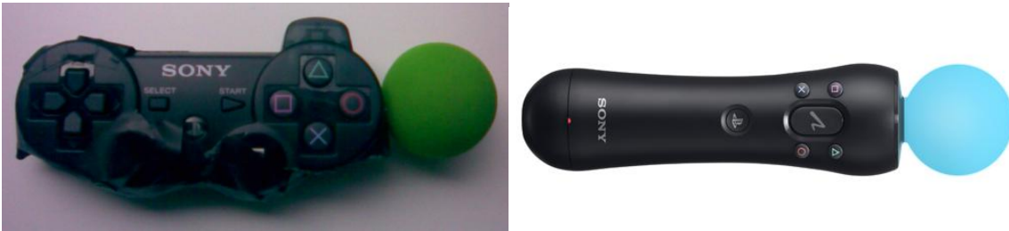
Figure 5. The PlayStation Move motion controller: initial prototype and final product.
