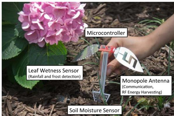
**Figure 1. Prototype of the inkjet-printed sensor SenSprout.**
