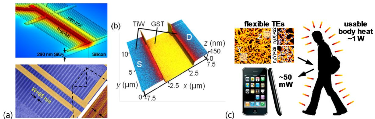
**Fig 1.** (a) Study of nanoscale heat flow in graphene revealed fundamental (ballistic) limits of phonon conduction in this 2D material [1,3,4]. (b) Thermal imaging of active PCM devices revealed key roles of thermoelectric effects at nanometer length scales [2]. (c) Flexible thermoelectrics (TEs) could be used to harvest power from the human body.
