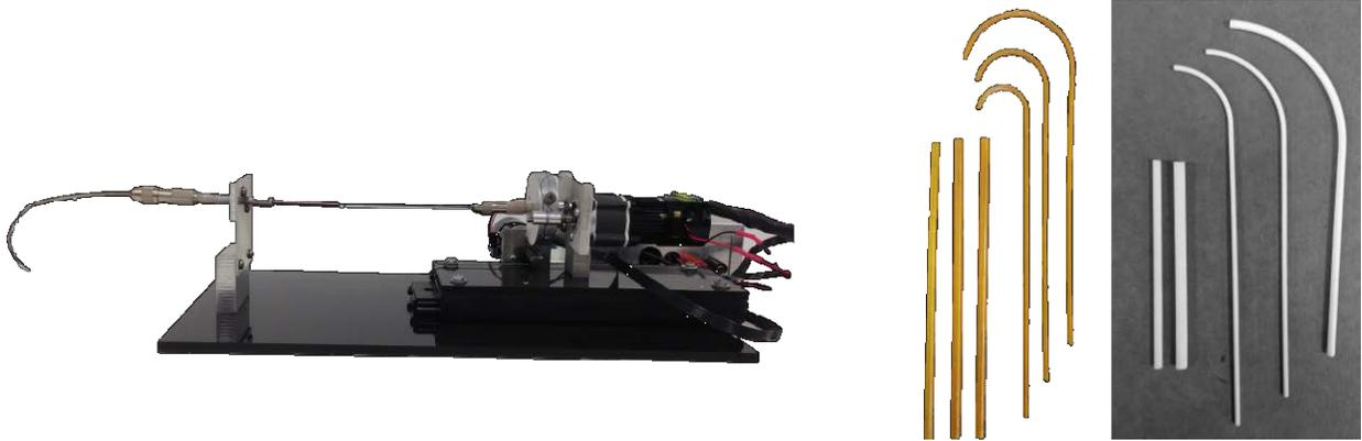
**FIGURE 2** (Left) Active cannula-driving robot module. (Right) Example sets of 3D-printed tubes that can be used to construct an active cannula system.
