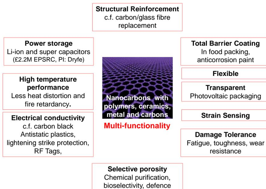
Figure 1: The potential applications of nanotubes and graphene in composites.
