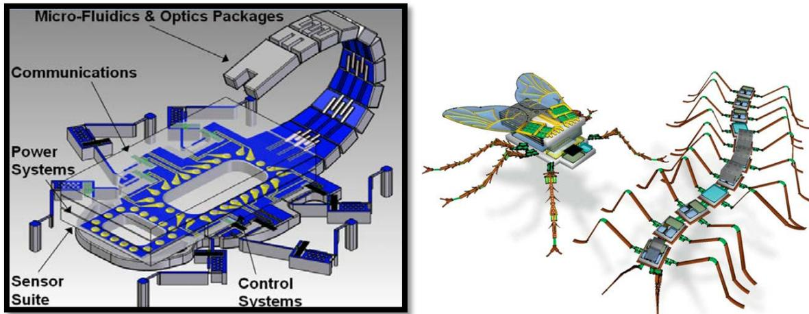
Figure 1. a) Notional mm-to-cm scale robotic systems based on a piezoelectric MEMS and a highly integrated microelectronics approach and b) illustration of notional ground and air mobile platforms.
