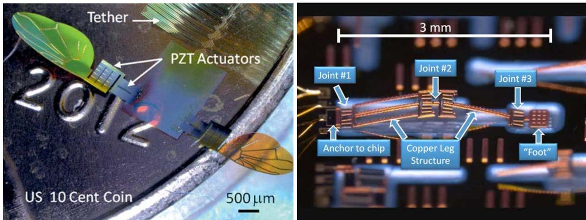
Figure 2. Examples of PiezoMEMS actuated microwings and a mm-scale robotic leg using PZT thin film actuators and multi-layer copper structural components
