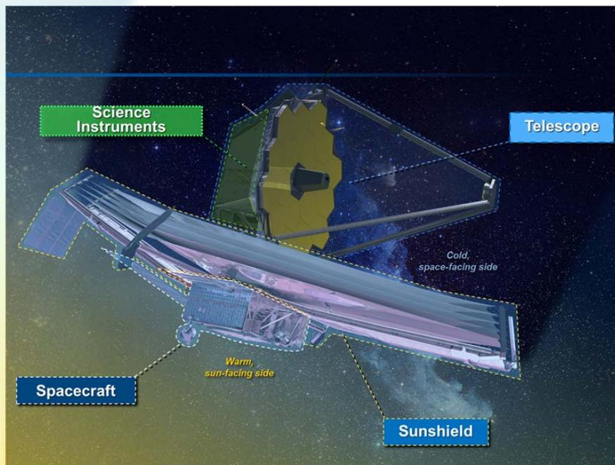
**Figure 3: Main Elements of JWST, with the tennis court sized Sunshield shading the Observatory from the intense solar radiation.**
